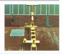
Heavy duplex model, Electroplated steel or stainless steel. Standard length: 1920 mm/ 75.6", 7 centering crosses. Suited for pipes from OD 324/12".
