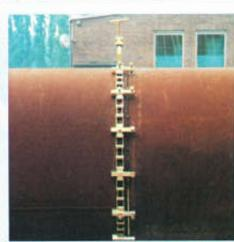
Examples: Photos of standard pipe-align chain. The same applications are possible with the short-linked version.
